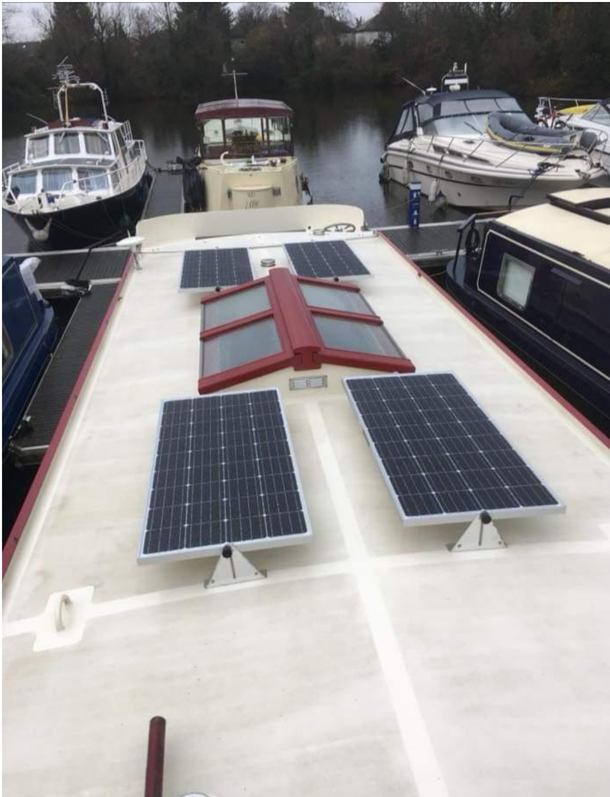
A 4 panel system on a wide beam Euro style cruiser, positioned around the huge ceiling skylight.
